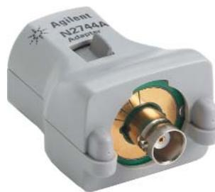
Also available is the N2744A T2A (Tektronix TekProbe® interface to Agilent AutoProbe) probe interface adapter. This adapter allows users of Tektronix TekProbe active probes to connect directly to the InfiniiVision 3000 X-Series AutoProbe interface BNC input. Protect your previous probe investment while taking advantage to the InfiniiVision 3000 X-Series' unique capabilities and value.
